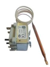
These devices automatically switch off the current in the controlled circuit as the pre-set temperature limit is reached, thus preventing overheating. Once the defection of the temperature regulation was repaired, in voltage-free state, the limiter / protective guard can be re-started manually.
